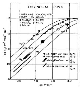
Using gases assumed to be efficient third bodies (CF<sub>4</sub> and SF<sub>6</sub>) the bimolecular reaction rate  $(k_{\Pi})$  dependence on the pressure of M was followed. The results when plotted in the Lindemann Hinshelwood form
